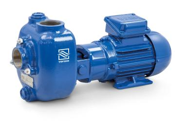
**Product Data** Suction port Threaded - 2" ISO 228 (BSP) Delivery port Threaded - 2" ISO 228 (BSP) Qmax 36 m<sup>3</sup>/h - 600 l/min (158 USgpm) Hmax 20 m (65 ft) Solids handling 17 mm (0.67 ") Motor power 1.5 kW - 2 HP Motor type **IEC** standard Winding for inverters **Cast iron frame** Motor brand WEG W22 Premium Weight 40 kg (88 lb)
